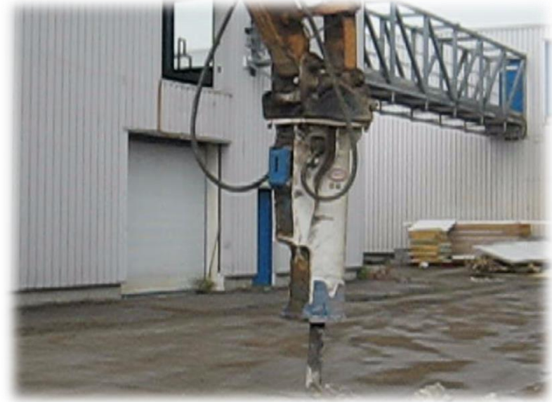
Installed Blank-Firing Protection System
